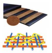
The multiply carcass is made of 2 to 4 plies, linked together by a layer of rubber. The interplies provide impact resistance to the structure of the belt and can also be oil and fat resistant and flame retardant.
